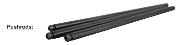
Isky Pushrods are One-Piece, 5/16" Diameter design and are manufactured from the finest grade available of Seamless .080" Wall, Chrome Moly Tubing. They are specially Heat Treated.
